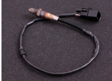
Fig 3.4.1b - Bosch wideband sensor. Not included if vehicle have factory mounted wideband sensor(s).
