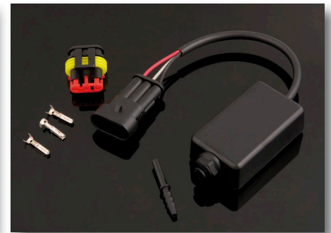
Fig 1f - External MAP-sensor can be used on analog input (0-5V) if internal (400kPa) is too small for ex. high boost applications (over 3bar boost) or back-pressure measuring. Optional and not included!
