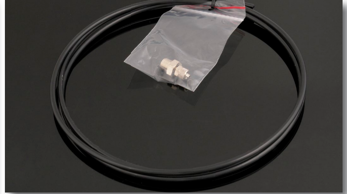
Fig 1c - Pneumatic hose and fittings. Used to connect MaxxECU's internal MAP-sensor to engine inlet manifold. If vehicle equipped with air flow meters, the MAP-sensor replaces it.
